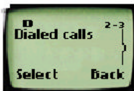
Figure 1. Mobile 'phone display showing sub-menu and navigation. Third sub-option of menu two displayed. The next level in the tree can be reached by pressing Select and the previous by Back.
